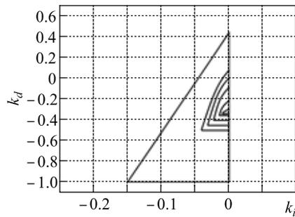
**Fig. 3.** Example 1. The boundaries of the  $H_\infty$ -controllers for different levels of  $\gamma$ .
