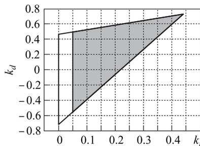
Fig. 5. Example 2. PID-controllers satisfying the direct criterion  $F < 0.1$ .
