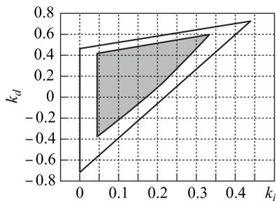
Fig. 4. Example 2.  $H_\infty$ -PID-controllers using the weight function.
