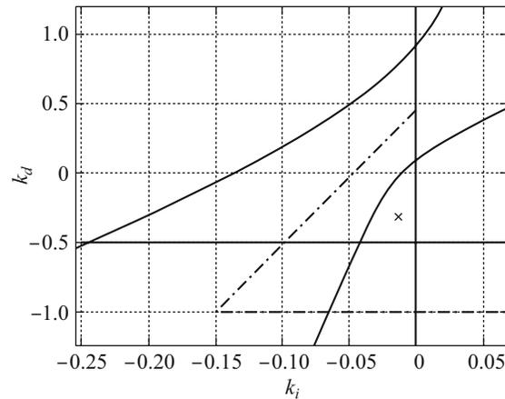
Fig. 6.  $H_\infty$  region for PID-controllers.
