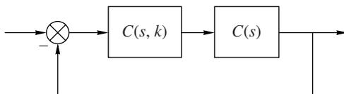
Fig. 5. Block diagram of the control system.
