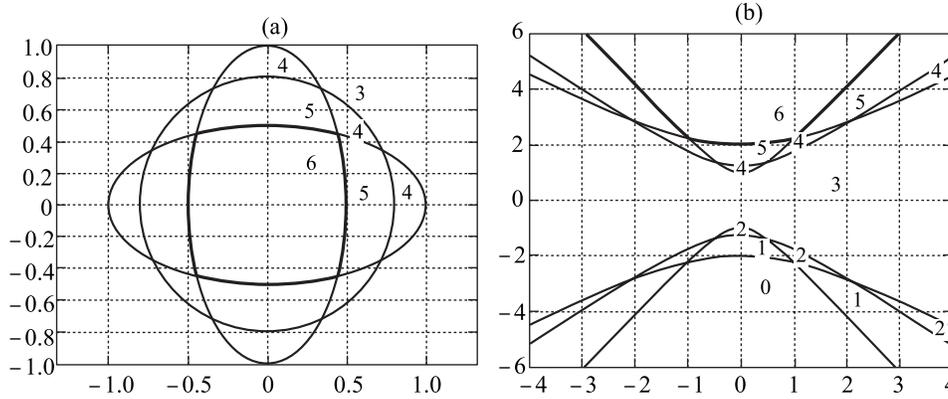
**Fig. 2.** Examples of  $D$ -decomposition for families (8) and (9) with  $b_1 = 1, b_2 = 1.25, b_3 = 2, c_1 = 2, c_2 = 1.25, c_3 = 1$ .
