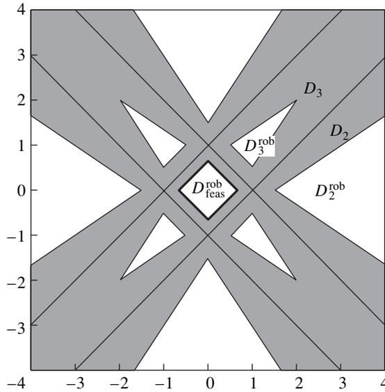
Fig. 8. Example of robust  $D$ -decomposition with respect to two parameters.
