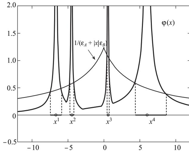
**Fig. 7.** Robust  $D$ -decomposition with respect to a single parameter, with uncertainty entering  $A$  and  $B$ .
