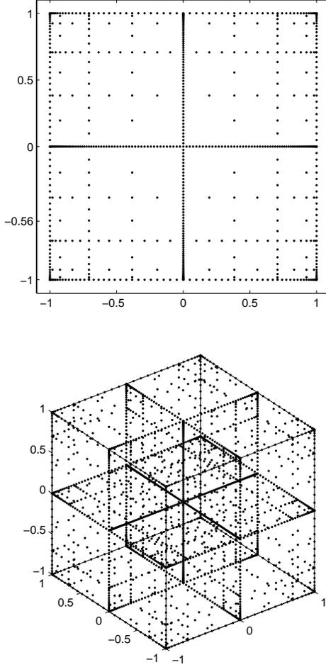
Fig. 1. Two and three dimensional sparse grids for  $\ell = 7$ . The number of grid points is respectively 705 and 2561.
