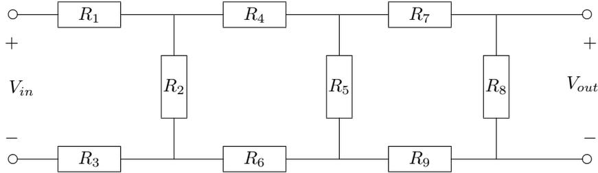
Fig. 2. Three-loop resistive ladder network.
